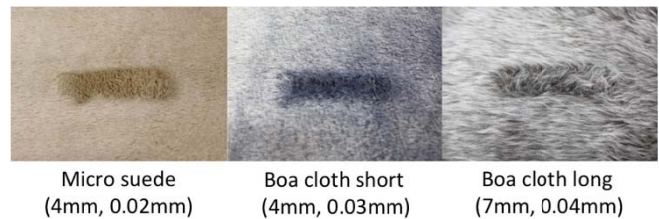
Figure 3: Materials used in the experiment. Numbers indicate fiber length and diameter.
