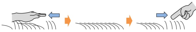
Figure 2: Principle of drawing on fur. Sweeping the fur surface in its growth direction flattens it, and sweeping it in the opposite direction raises it.
